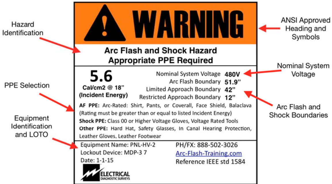
Figure 2 – NFPA 70E – 2015 Compliant Arc Flash Label
