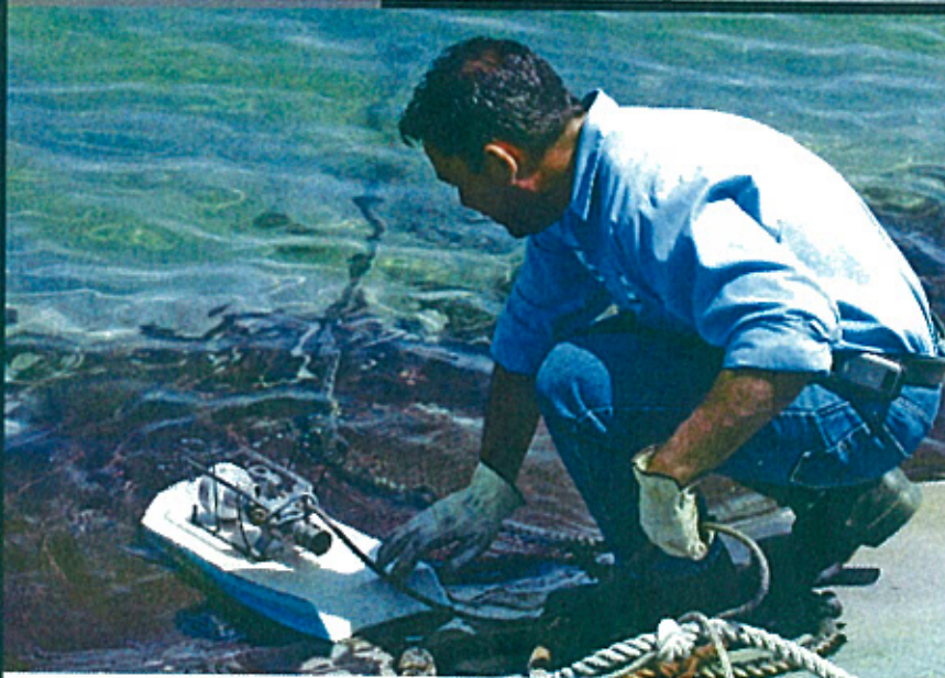
Chris Lopez cut the 36- by 30-inch Boogie board to fit a 12-inch PVC pipe and tested it on the district's recycled water detention basin. (Photos courtesy of Rancho California Water District)
